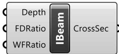
Figure 57 - The I-Beam (IBeam) component
